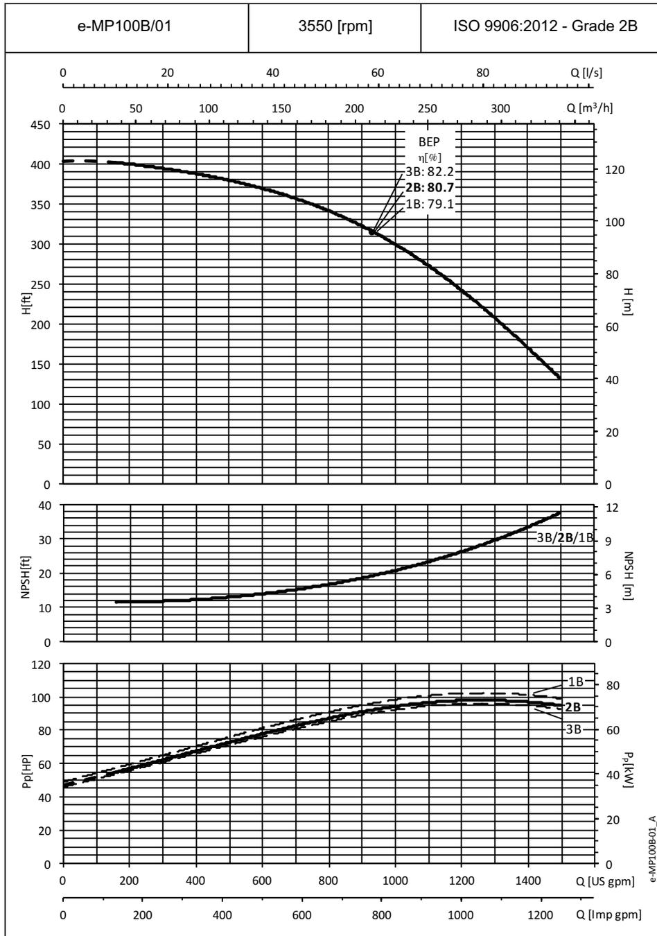
The example above summarizes differences in the published performance based on three different acceptance grades (1B, 2B and 3B). Different tolerances allowed between the published and the actual efficiency (-3% for Grade 1B, -5% for Grade 2B and -7% for Grade 3B) could be misleading when acceptance grade is not considered in the assessment of a pump performance.
